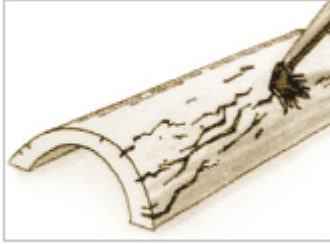
Use slip to fill small cracks that can appear as the piece dries.
